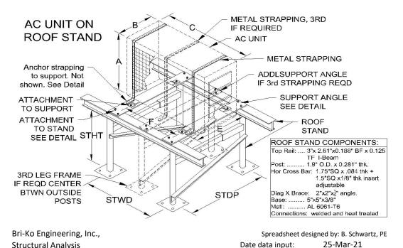
Calc Sht: EC-1 Mechanical Equipment on Roof Stand Calc
